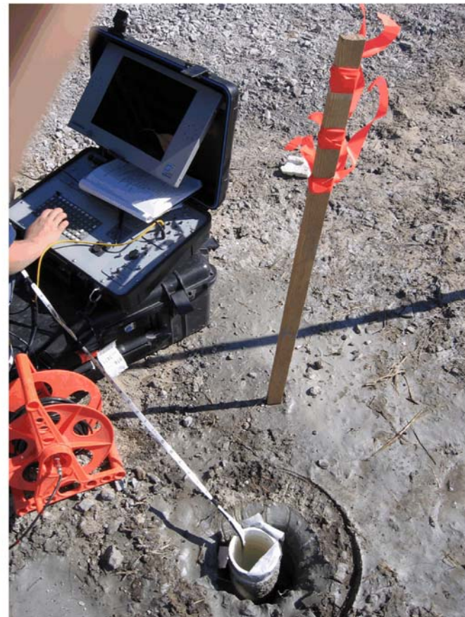
Figure 2 - Photographs of impacting Wall of IHNC Levee at South Borehole of South Breach and Freedom Data PC at Cased Borehole with Hydrophone Receiver Downhole
