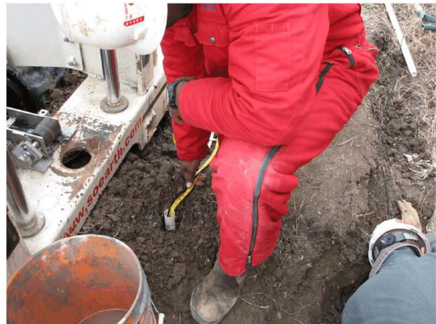
Photo 10 - Small Hydrophone receiver on tape in 1 inch PVC casing installed by Geoprobe Rig at IHNC
