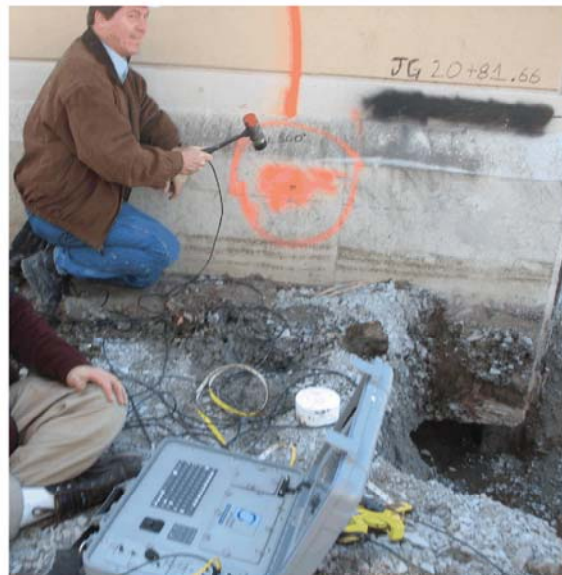
Photo 5 (Fig. 3) - Angled downward impact to chamfer of wall at ~ el. 5.75
