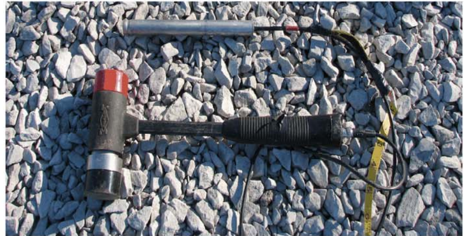
Photo 8 - 3-lb Impulse Hammer with black hard plastic tip and small diameter hydrophone used in PS re-tests
