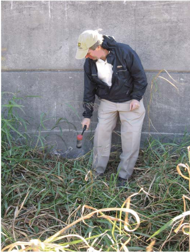
Figure 2 - Photographs of impacting Wall of IHNC Levee at South Borehole of South Breach and Freedom Data PC at Cased Borehole with Hydrophone Receiver Downhole
